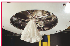
Cinch spouts concentrically with POWER-CINCHER® flow control valve*
