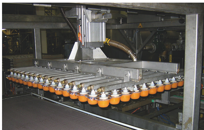
Cups leaving the filler/sealer are transferred to retort trays by vacuum grippers. Each tray holds 192 cups.
