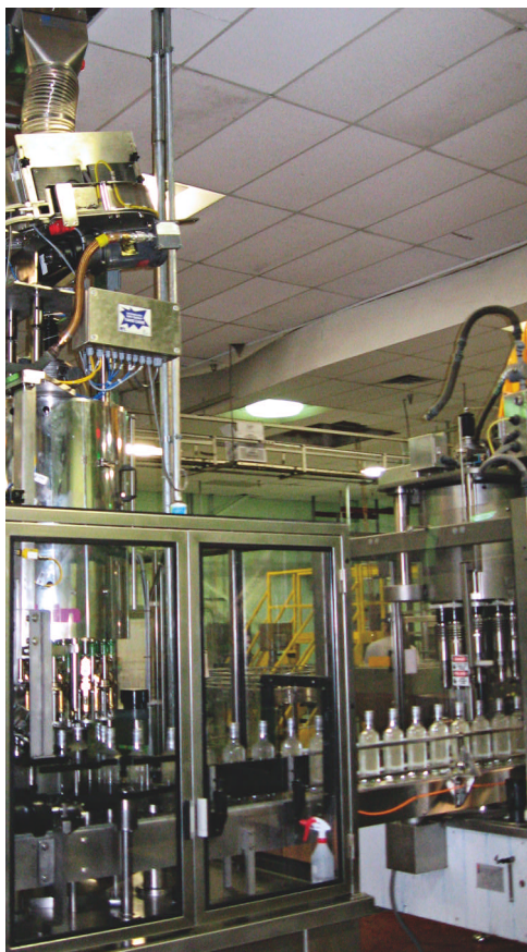
A new rinser/filler/capper tribloc runs 300 bottles of liquor/min. The rinser and filler transport bottles by grippers beneath the neck, which minimizes chipping. In the 10-head capper, individual sealing heads descend onto the bottles with a 200-lb top load force to seal the caps onto the tops of the bottles.
